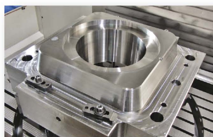
11 ltr pail cavity during milling operation
